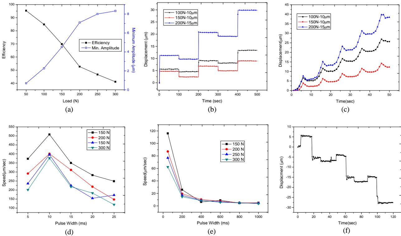
Fig. 7 Performance of nanopositioner a) efficiency and minimum displacement for the nanopositioner b) forward motion with a square signal c) forward motion with a triangle signal d) dynamic performance with short pulse width e) dynamic performance with long pulse width f) backward motion of the nanopositioner
