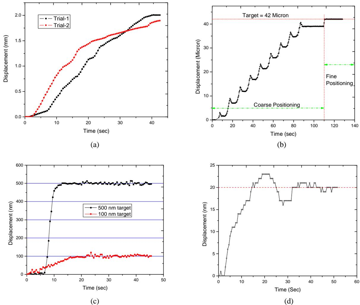
Fig. 8 Performance of nanopositioner a) Long range positioning b) Hybrid positioning c) Fine positioning d) Minimum resolution performance
