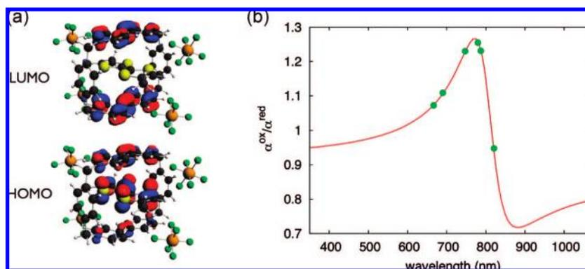
**Figure 5.** (a) The HOMO and LUMO for the TTF-CBPQT•4PF<sub>6</sub> complex. The CT transition responsible for the absorption at 820 nm is a result of a transition from the HOMO on TTF to the LUMO on CBPQT<sup>4+</sup>. (b) TDDFT-calculated polarizability ratio between the two states of  $2^{4+}$  as a function of wavelength. The solid line is a fit to the calculated values using a one-oscillator Lorentz model.
