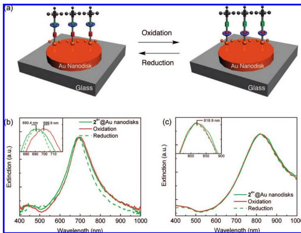
**Figure 2.** (a) Schematic of working principle of the molecular-machine-based active plasmonics. (b) Extinction spectra recorded from  $2^{4+}$ -derivatized Au nanodisks in air with an initial peak wavelength of  $690.4 \pm 0.2$  nm during the redox process. (c) Extinction spectra recorded from  $2^{4+}$ -derivatized Au nanodisks with an initial peak wavelength of  $818.9 \pm 0.2$  nm during the redox process. Insets in (b) and (c) are expanded views around the peak maxima in the spectra.
