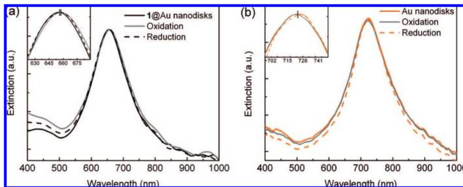
**Figure 3.** (a) Extinction spectra recorded from **1**-attached Au nanodisks in air during the redox process. A very small peak shift was observed during the redox process. (b) Extinction spectra recorded from bare Au nanodisks. No obvious peak shift was observed during the redox process. Insets in (a) and (b) are expanded views around the peak maxima in the spectra.
