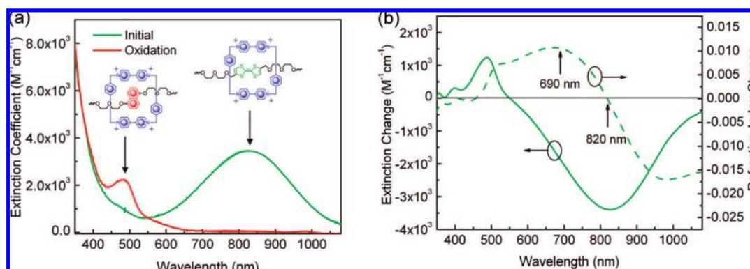
**Figure 1.** Extinction spectra and refractive-index change of **2<sup>4+</sup>** in solution: (a) The extinction spectra of **2<sup>4+</sup>** in DMF (0.05 mM) before (green line) and after (red line) oxidation by 2 equiv of Fe(ClO<sub>4</sub>)<sub>3</sub>. (b) The oxidation-induced refractive-index change (dashed green line) of **2<sup>4+</sup>** was derived from the differential extinction spectrum (solid green line) by using the Kramers–Kronig relation.
